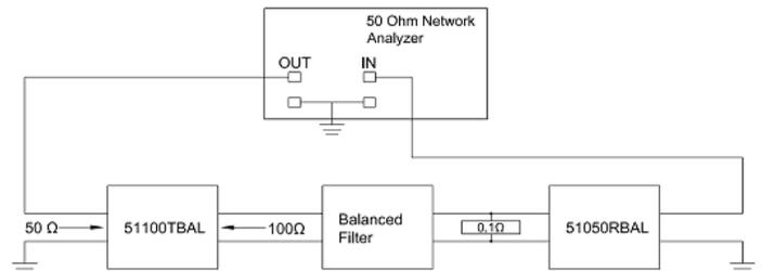
Figure 2. CISPR 17 Balanced 100Ω/0.1Ω Test Setup
