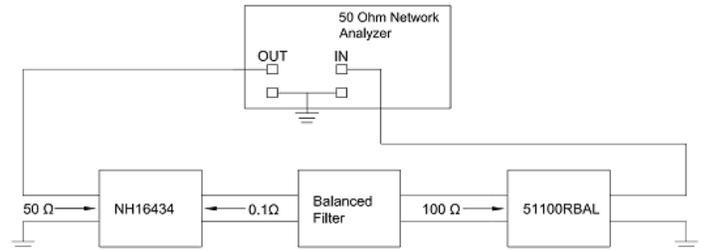
Fig. 1. Transformer-Coupled Data Bus Coupler Schematic.
