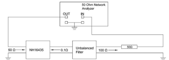
Figure 3. CISPR 17 Unbalanced 0.1Ω/100Ω Test Setup
