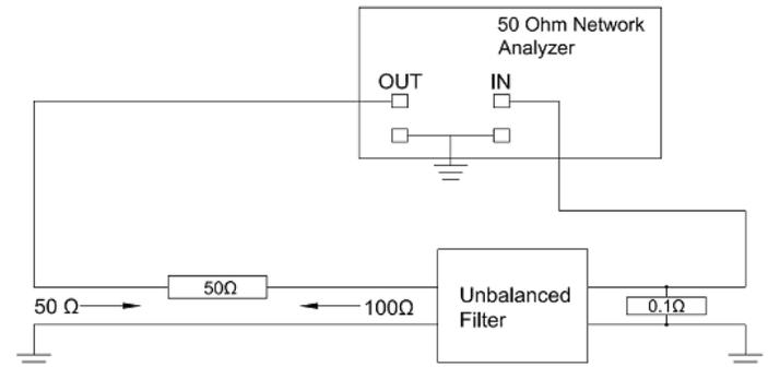
Figure 4. CISPR 17 Unbalanced 100Ω/0.1Ω Test Setup
