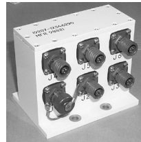
Fig. 9. Coupler for armor. Uses MIL-G-3899 connectors. Used on M1A2, tank.
