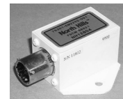
Fig. 2. 2-stub coupler with multi-pin connectors. Used on F-15E.
